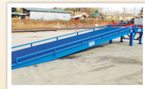
LOADING & UNLOADING RAMP
