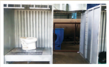
GREEN PIECE INSPECTION BOOTH WITH DUST EXTRACTOR
