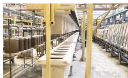
BEAM CASTING MACHINE WITH HEATING SYSTEM
